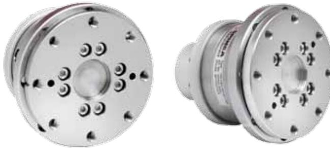
The RotoSpin rotary modules with type designation **A** are called flange ones. They feature a flange design, which allows the module's attachment and building into a structure with a circular hole. According to their size, RotoSpins A are manufactured in four size categories with load capacities of 60, 250, 500, and 1000 kg respectively.
