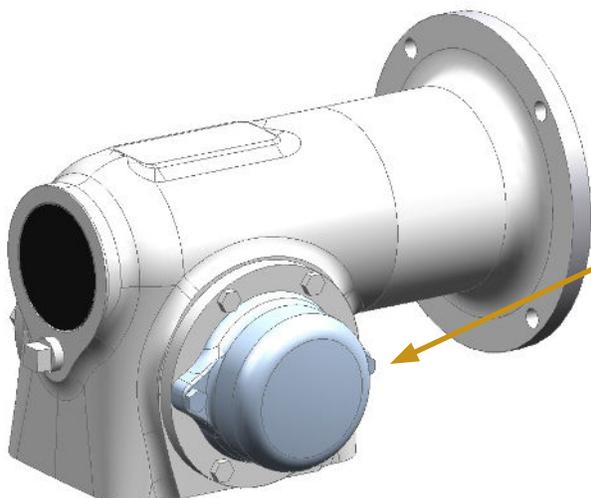
MOUNT THE COVER. INSTALL THE LENGTHENED CARRIER BOLTS PROVIDED. TORQUE IN ALTERNATING PATTERN TO:
