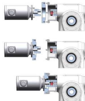
MOUNT THE MOTOR'S COUPLING HALF ON THE MOTOR SHAFT. POSITION TO THE DIMENSION SHOWN FOR THE APPROPRIATE ASSEMBLY.
