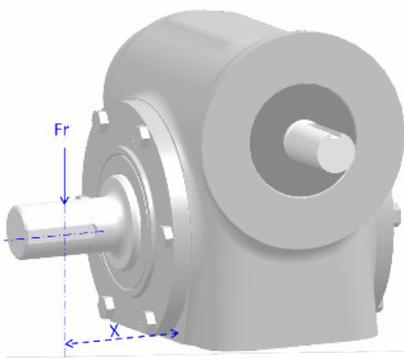
$$Fr = \frac{P \times 126,000 \times K}{n \times PD} \quad \text{OR} \quad Fr = T \frac{2}{PD} \times K$$
